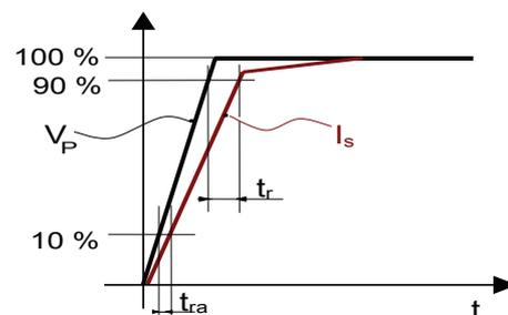
Figure 18: *response time  $t_r$  and reaction time  $t_{ra}$*
