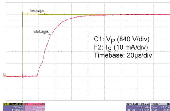
Figure 6: Typical step response (0 to 4200 V)
